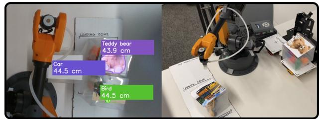
**Figure 2:** The MaskRCNN object detection framework displaying coordinates of objects relative to the Mirobot robot (left) and the robot sorting the objects (right).
